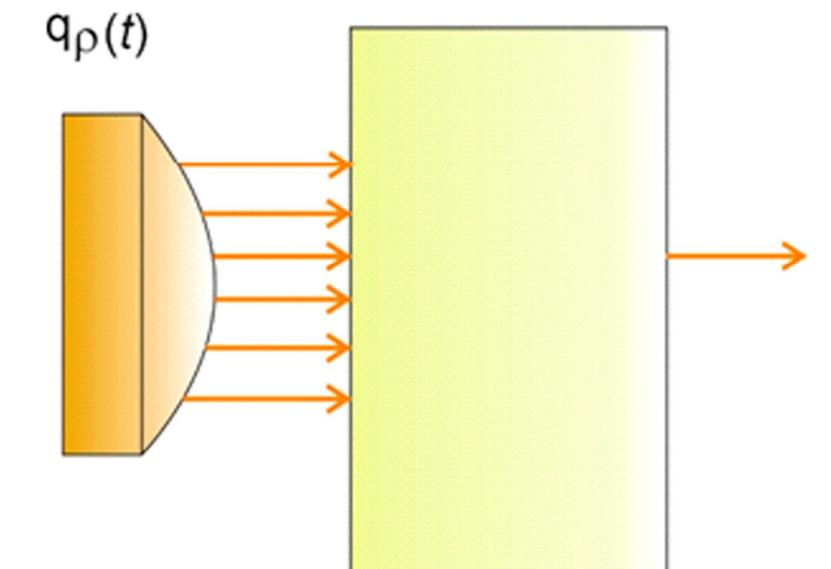
Thermophysical properties of carbon nanomaterials of various origins, including CNTs obtained by the CVD method, were studied using the impulse method of measuring thermal conductivity. Table shows the solution to the problem of thermal diffusivity calculation.
