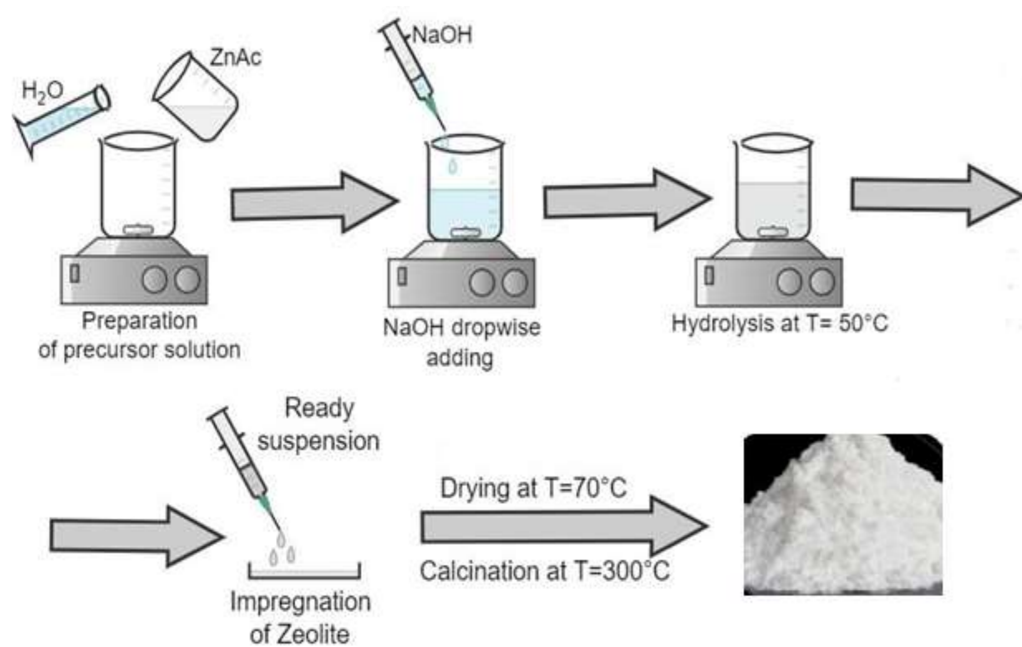
Fig. 1 – The synthesis scheme of ZnO/Zeolite composite.
