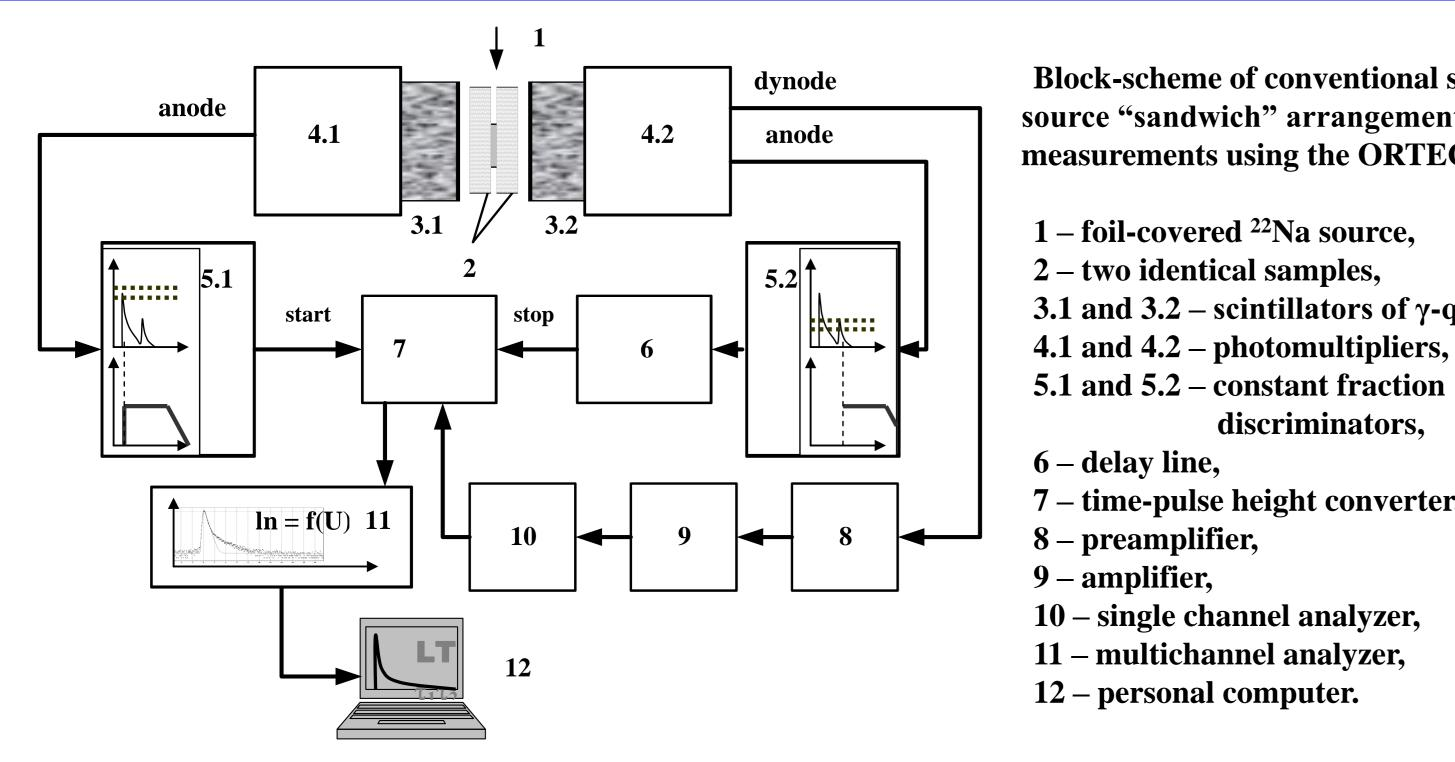
**Block-scheme of conventional sample**source "sandwich" arrangement for PAL measurements using the ORTEC apparatus:
