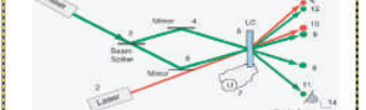
Fig. 5. Optical scheme of two-wave mixing in LC cell "Green" laser (second harmonic Nd:YAG) - for dynamic grating and self-diffraction of laser beams. "Red" laser (He-Ne) - for testing - diffraction on a given grating.
