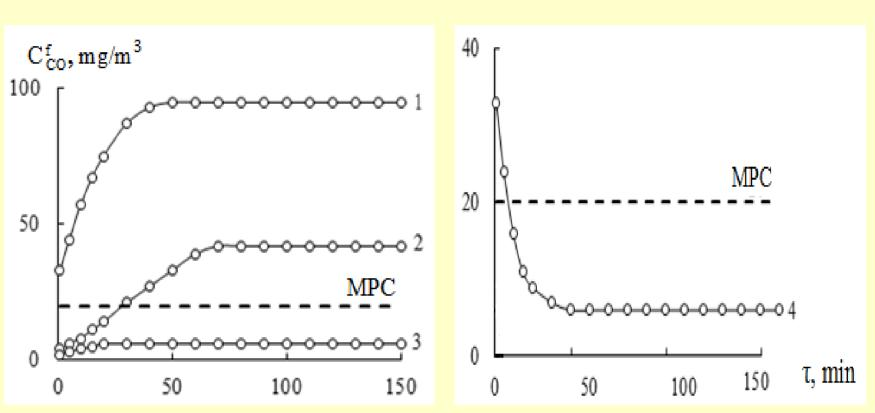
Dependence of the final CO concentration on time  $\tau$  in the oxidation reaction of carbon monoxide with atmospheric oxygen in the presence of a catalyst  $K_2PdCl_4$ -Cu( $NO_3$ )<sub>2</sub>-KBr/ $\overline{S}$ .  $\overline{S}$ : I-1H-TS-Phl-1; 2-2H-TS-Phl-1; 3-3H-TS-Phl-1; 4-6H-TS-Phl-1.
