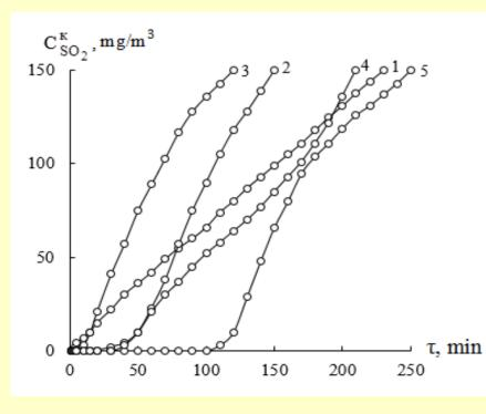
Dependence of the final concentration  $SO_2$  on time  $\tau$  in the reaction of oxidation of sulfur dioxide with air oxygen in the presence of the composition Pd(II)-Cu(II)- $KBr/\overline{S}$
