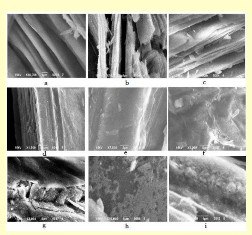
SEM images of samples of natural (a), thermally expanded (b, c) and acid-modified phlogopite (d-i).
