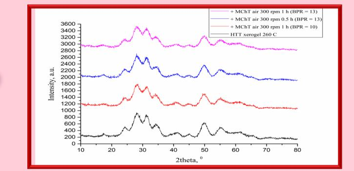
HTT forms developed mesoporous structure that is slightly changed due to next MChT in both cases
