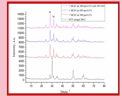
pH 7: HTT of wet gel at 300 °C for 5 h leads to formation of pure high-crystalline MP and phase composition does not change after next MChT
