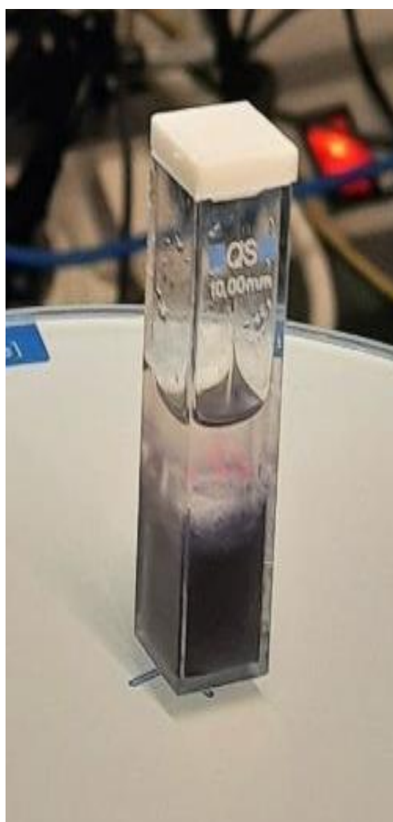
Fig. 4. Synthesis of Au NPs on ZnO by photo-deposition
